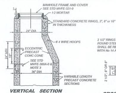
2 1/2" RINGS SHALL BE REINFORCED WITH TWO 1/4 ROUND STEEL HOOPS, 6" AND 8" RINGS SHALL BE REINFORCED WITH FOUR HOOPS, TIED WITH No 14 A.S. & W. GAUGE WIRE, 8" OC
