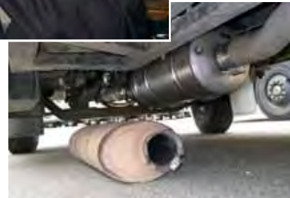
Installing a diesel particulate filter (DPF) in this Atlanta school bus simply required removal and replacement of the muffler and tailpipe.
