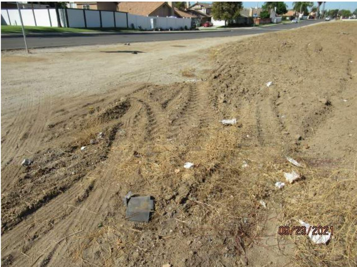
**PHOTO 10** - Southwesterly view looking down in an area in relative close proximity to the southeast corner of the subject site. In the lower portion of the photograph, obscured by weeds or vegetative debris is a small area of heavy hydrocarbon-stained soils, possibly including waste and/or hydraulic oils. Another such area, round in shape, is evident towards the top of the photograph, shown in the dirt area near the Copper Cove Lane roadway.
