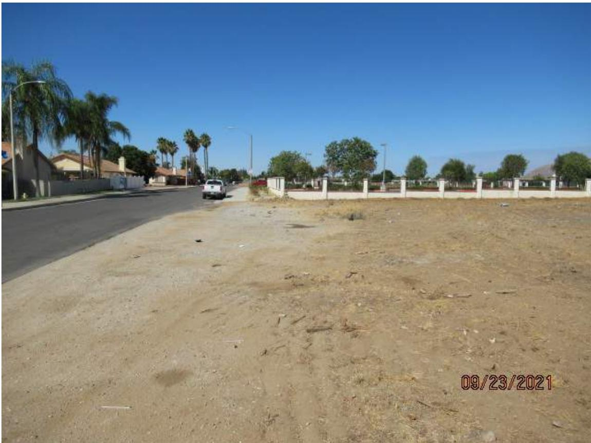
**PHOTO 14** - View facing west along the south subject site boundary and right-of-way for Copper Cove Lane, looking towards the southwest corner of the subject site. At the photograph center and in lower areas near the roadside are small areas of heavy hydrocarbon-stained soils, such as from waste oil. These stained soils are anticipated to be surficial or near surface in vertical extent.
